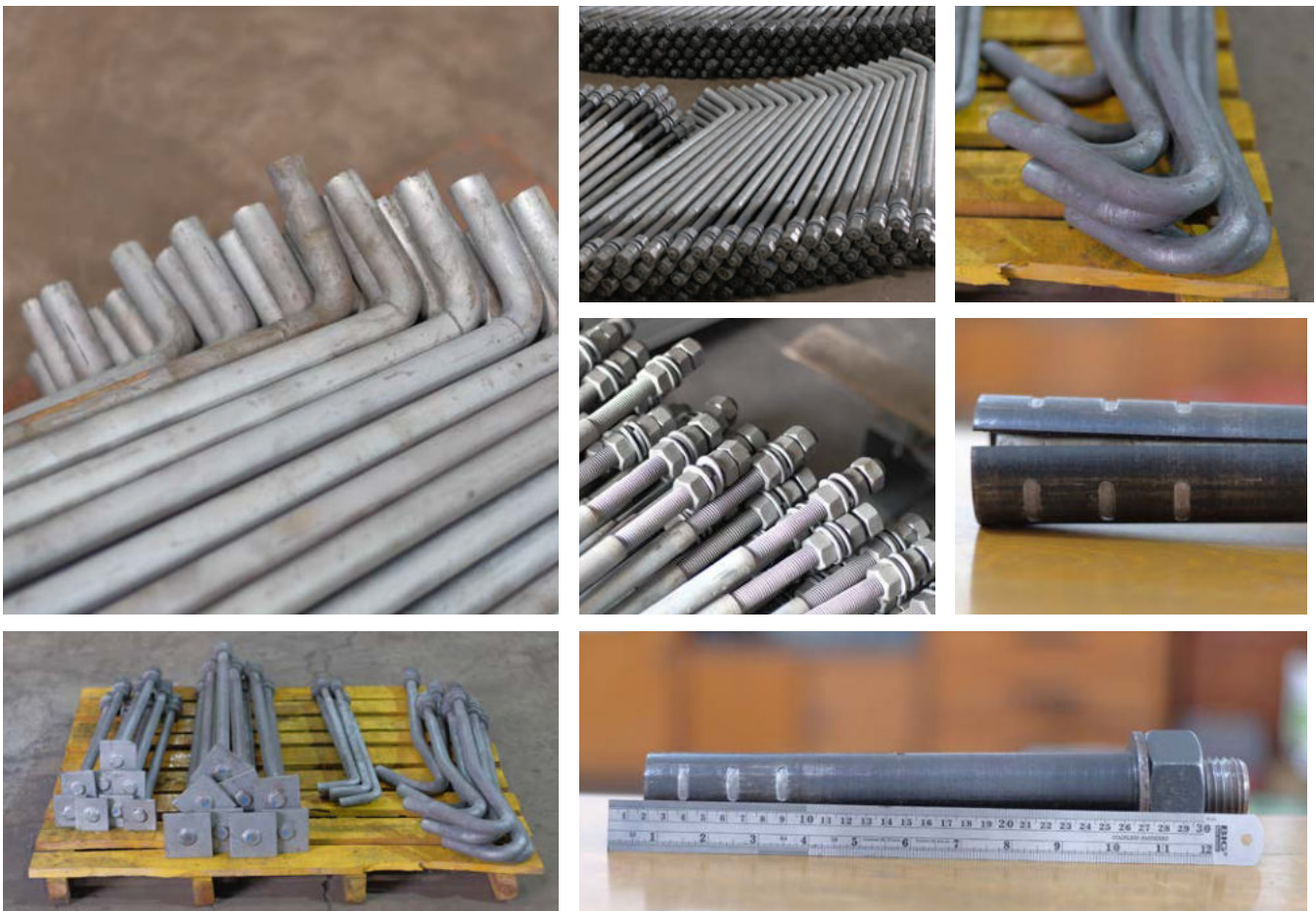
Customize expansion bolt until maximum diameter 150mm, length maximum 3m, material (ST41 up to ST60), Carbon Steel (SUS 304 up to 316), Stainless Steel. Various customized anchor (S45C) / expansion bolt with grade ST41/ ST60 carbon steel , an galvanizing ) or SUS304.
